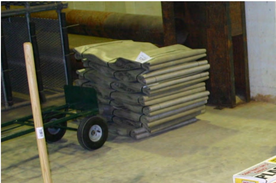
Figure 5. A stack of Geocells. Each bundle is two units of 16-ft-long lengths.
