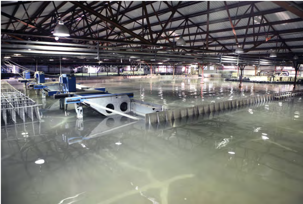
Figure 1. Research basin with wave machines on the left side and the test area on the far right. The test area is shown in closer view in Figure 2.
