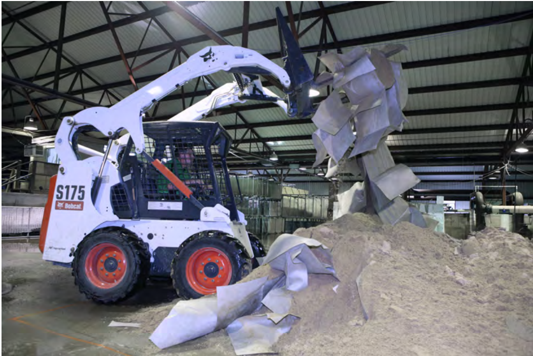
Figure 61. As the fabric is lifted, the sand separates from the cells.
