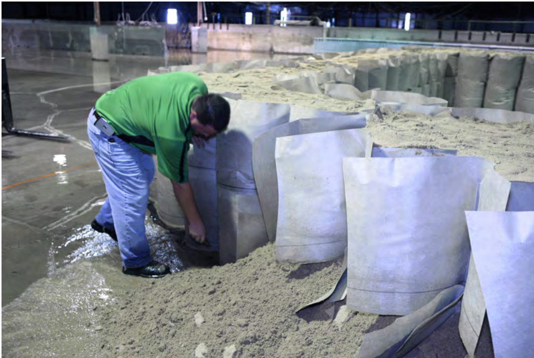
Figure 59. Geocells are sliced open with a box cutter for removal.
