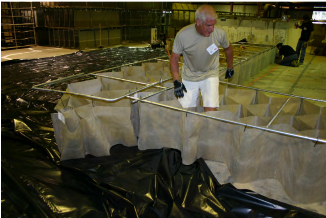
Figure 10. The unit on the left has been shortened to fit the designated area for the test. The extra cells will be cut off with a box cutter.
