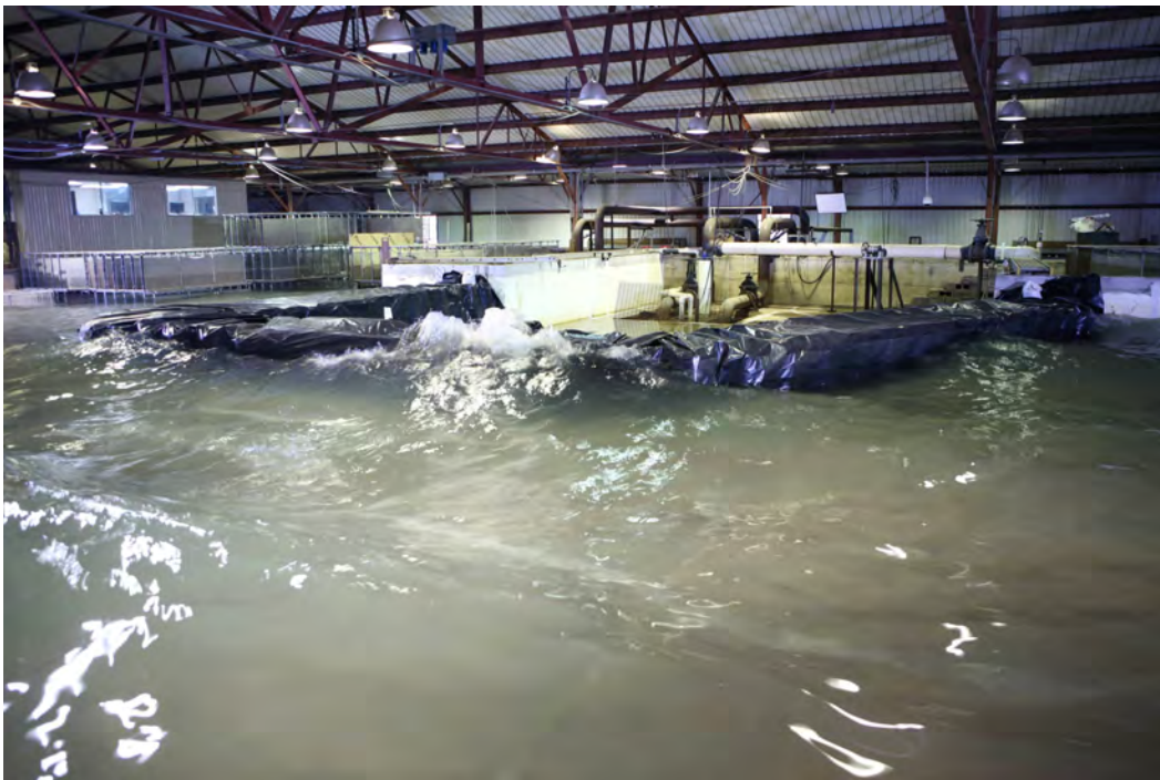
Figure 2. Test area surrounded by a Typar® Geocell barrier, viewed from the test basin. The measurement sump and pumps are in the back of the test area.
