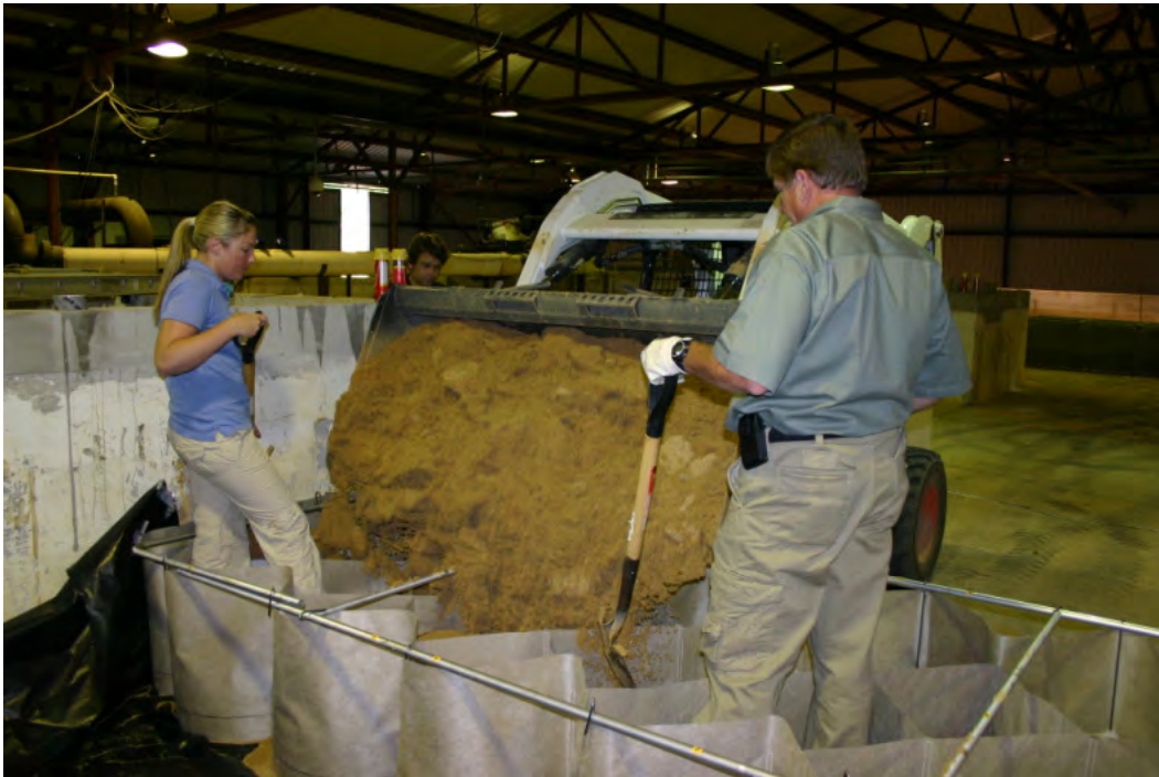
Figure 11. Sand being dumped into the Geocells.
