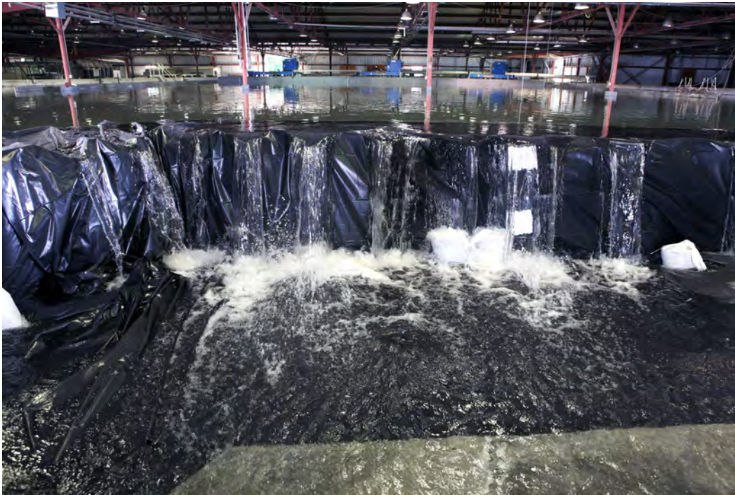
Figure 50. Flow over the barrier during the overtopping test.
