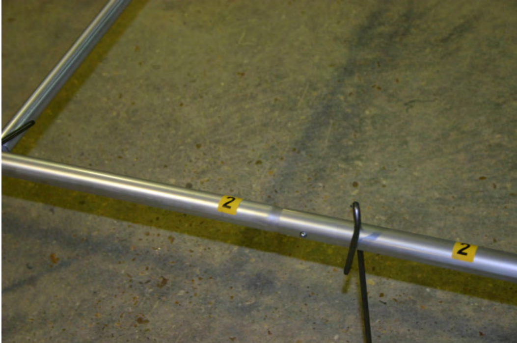
Figure 7. Framework parts are numbered at each connection for easy reference. The push-pin connecting two lengths of tubing is visible near the middle of the picture.
