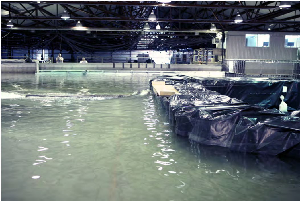
Figure 53. Debris impact test with log towed into the barrier.
