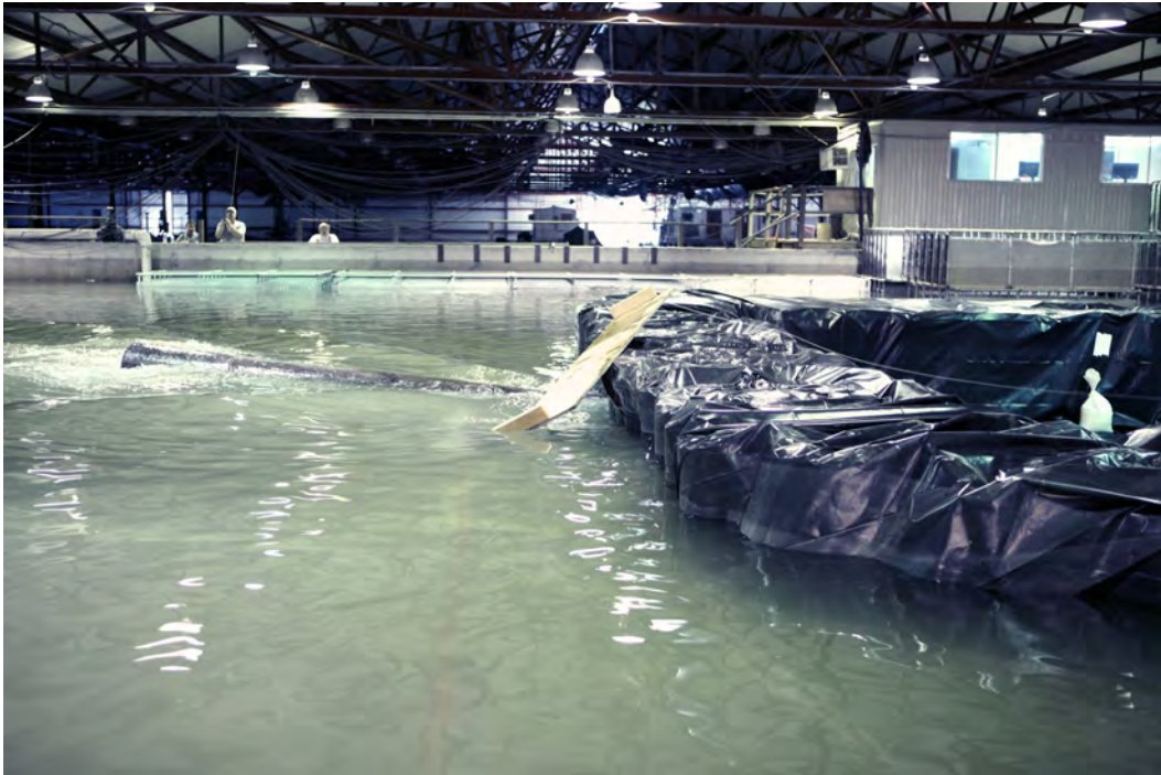
Figure 54. Debris impact test as log struck barrier.
