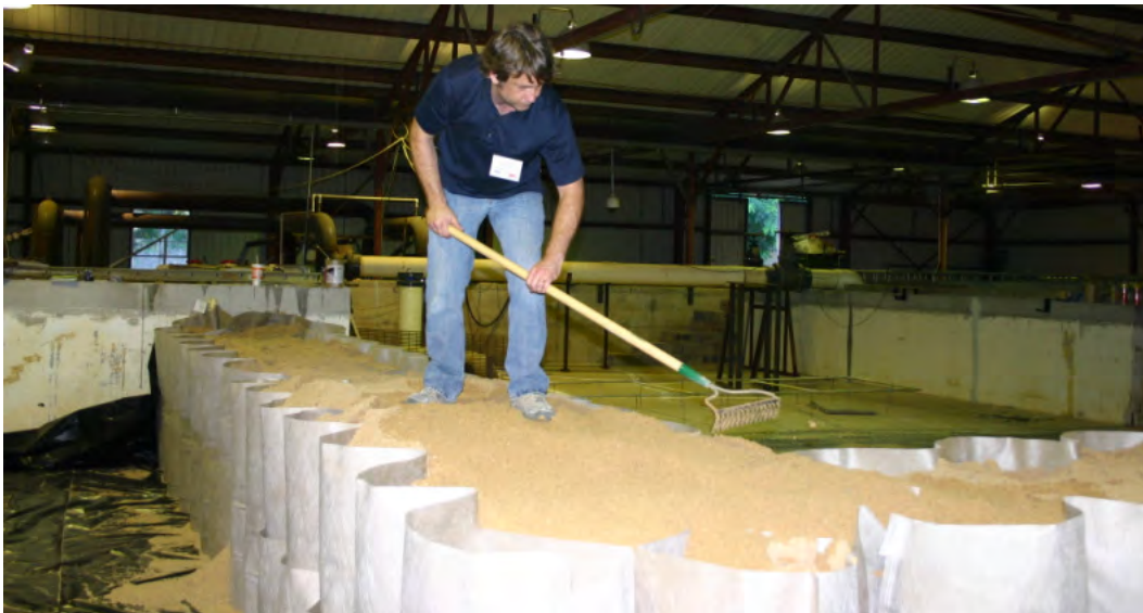
Figure 18. Leveling the top of the barrier.
