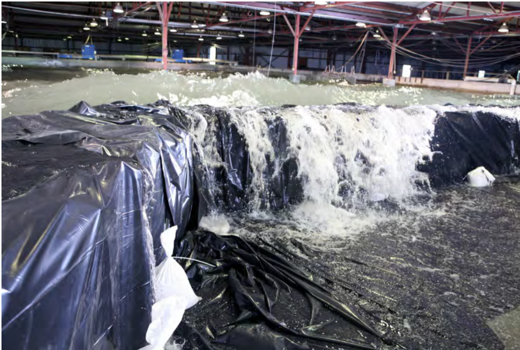
Figure 47. Wave overtopping during test with high water, large waves.
