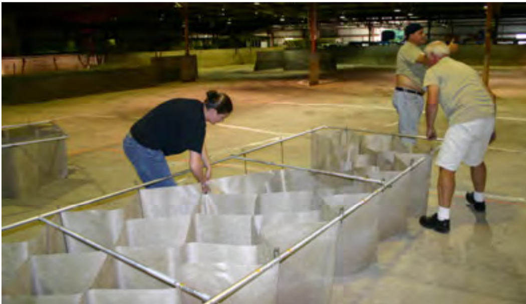
Figure 8. Aluminum framework holding open a length of Geocells.
