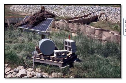
Debris on top of the solar panel indicates the high watermark from the 1,000-year rain event.
